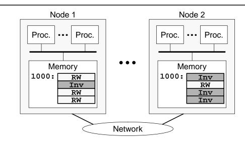
**Figure 2-4.** Stache example, step 3. Node 2 has fetched a block of data from node 1 to satisfy the store access. In this example, node 2 obtains exclusive access to that block and node 1's copy is marked invalid. To satisfy a read access, node 2 would obtain a read-only copy, leaving node 1 also with a read-only copy.
