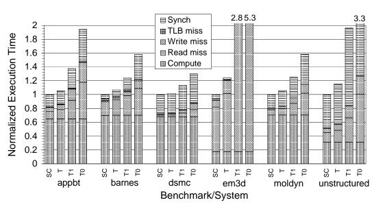
**Figure 3-13.** Execution time breakdown for transparent shared memory. SC=Simple COMA, T=Typhoon, T1=Typhoon-1, T0=Typhoon-0.
