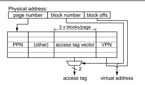
**Figure 3-6.** Typhoon RTLB diagram. Arrows indicate how a physical bus address is processed by the RTLB to generate the block's access tag and virtual address. The handler table pointer, user data pointer, and home node ID RTLB fields are not shown. The PPN field holds the physical page number; VPN is the virtual page number.
