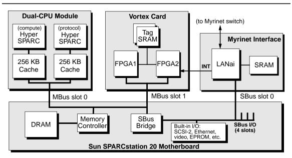
**Figure 4-1.** Block diagram of a Typhoon-0/COW node. The Myrinet LANai chip integrates a simple processor, a DMA engine, network transceivers, and most of the bus interface logic.
