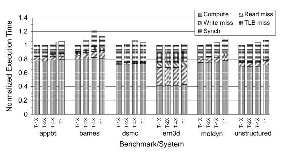
**Figure 3-19.** Execution time for the application-specific protocols on Typhoon, varying the protocol processor speed. T-nX=Typhoon with protocol CPU n times slower than compute CPU, T1=Typhoon-1. Network latency is 0.5 µs.
