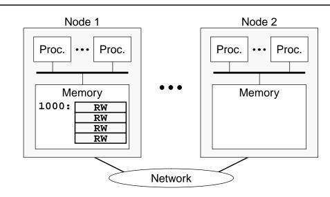
**Figure 2-2.** Stache example, step 1. Node 1 is the home node for the page at virtual address 1000. Node 1's processors have read-write access to all the blocks on the page (indicated by the **RW** label on each block). Node 2 has no mapping for virtual address 1000.
