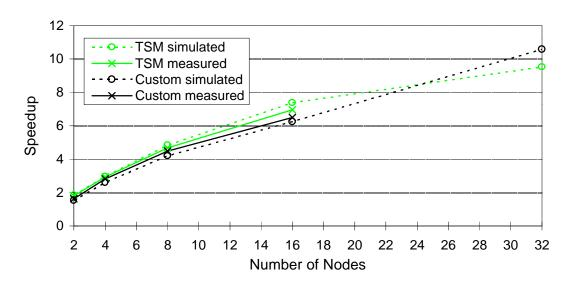
Figure 4-4. Simulated and measured speedups for Barnes.
