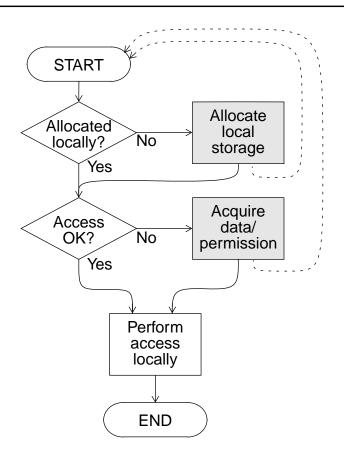
**Figure 2-1.** DSM memory access flowchart. If either the allocation check or the access check fails, the system must take action before the reference can be performed. The solid arrows indicate that the reference is suspended and later resumed without repeating the allocation and access checks. An alternate approach is to abort and retry the reference, as indicated by the dotted arrows.
