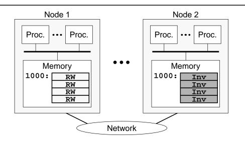
**Figure 2-3.** Stache example, step 2. Node 2 has mapped a memory page at address 1000 in response to an access from one of its processors. Because node 2 has no valid data for the page, the blocks on the page are marked invalid using the fine-grain access control mechanism (indicated by the **Inv** label on each block).
