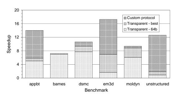
Figure 4-2. Application speedups on 16 nodes of the prototype system.
