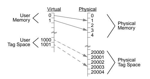
**Figure 3-4.** Shadow tag space example. The hardware device interprets accesses to physical tag space page 2000x as tag operations on physical memory page x. The user program requests operations on its virtual page y by accessing its virtual page 100y. The shadow mappings (dashed arrows) dual the memory mappings (solid arrows), implicitly translating the address component of the user's requests.
