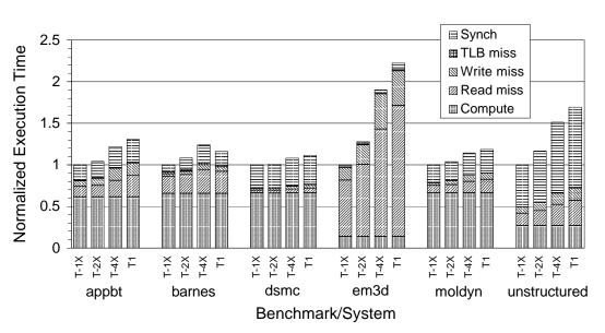
**Figure 3-18.** Execution time for transparent shared memory on Typhoon, varying the protocol processor speed. T-nX=Typhoon with protocol CPU n times slower than compute CPU, T1=Typhoon-1. Network latency is 0.5 µs.
