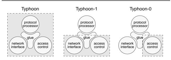
**Figure 3-3.** Component integration diagram. For each system, a shaded rectangle indicates the components integrated into custom hardware.
