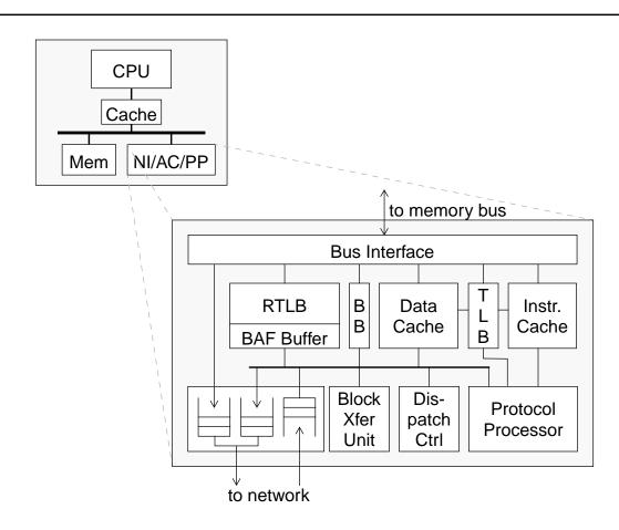
**Figure 3-5.** Typhoon node, including a block diagram of the network interface/access control/ protocol processor device. RTLB is the reverse TLB; BB is the block buffer; the BAF buffer holds information on block access faults. The second network send queue is for use by the compute processor(s).
