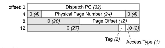
**Figure 3-8.** Dispatch register layout for block access faults. Parenthesized numbers are field widths in bits. The access control device aligns fault information to accelerate the handler dispatch code (see Figure 3-9). Because this register is cacheable, these four words are transferred in a single bus transaction.
