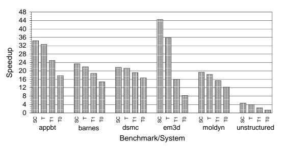
**Figure 3-12.** Application speedups for transparent shared memory on 32-node systems. SC=Simple COMA, T=Typhoon, T1=Typhoon-1, T0=Typhoon-0.
