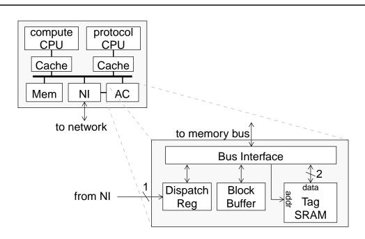
**Figure 3-11.** Typhoon-0 node, including a block diagram of the access control device. The device's control logic is not shown. The network interface is shown on the memory bus, but may be attached to an I/O bus instead.
