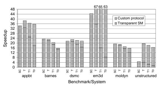
**Figure 3-14.** Application speedups on 32-node systems, including application-specific protocols. SC=Simple COMA, T=Typhoon, T1=Typhoon-1, T0=Typhoon-0.
