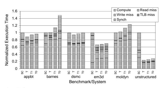
**Figure 3-15.** Execution time breakdown for the application-specific protocols, normalized to transparent shared memory on Simple COMA. SC=Simple COMA, T=Typhoon, T1=Typhoon-1, T0=Typhoon-0.
