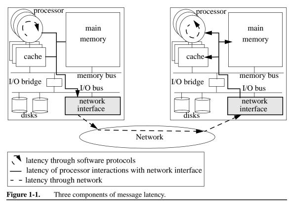
• latency of processor interactions with a *network interface (NI)* that connects a computer with a network.
