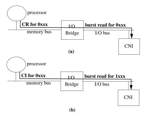
**Figure 3-5.** Illustration of shadow address with a CNI on the I/O bus. (a) a processor read miss (CR = coherent read) for the address 0xxx is translated by the bridge to a burst read for 0xxx on the I/O bus. (b) shows that a CI (coherent invalidate) signal for 0xxx is translated to a burst read for the shadow address 1xxx. The CNI interprets a read for 1xxx as a invalidation signal for 0xxx.
