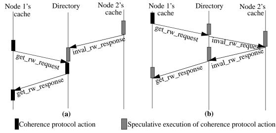
**Figure 6-4.** Two examples of using prediction to accelerate coherence protocols. (a) shows a protocol in which protocol actions are accelerated in anticipation of Node's 1 write miss. (b) shows a protocol that predicts incoming coherence messages, updates protocol state, generates (but does not send) messages speculatively, and commits protocol state and messages only if the predicted message arrives.
