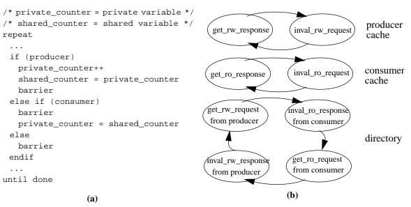
**Figure 6-2.** Message signature generated by a producer-consumer sharing pattern. (a) shows a pseudo code for the producer-consumer sharing pattern. A producer writes to a shared counter and a consumer reads the shared counter. (b) shows the sequence of messages received by the producer cache, consumer cache, and directory for the cache block containing the shared counter (assuming no false sharing). Table 6.1 explains the different message types shown in this figure.
