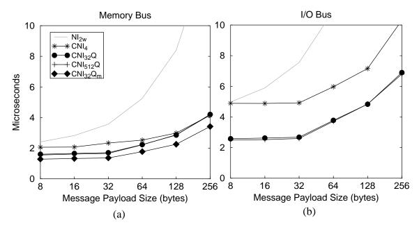
**Figure 4-1.** Process-to-process round-trip message latency. This figure shows the process-toprocess round-trip message latency in microseconds (vertical axis) for different message sizes (horizontal axis). (a) shows the round-trip message latency for  $NI_{2w}$ ,  $CNI_4$ ,  $CNI_{32}Q$ ,  $CNI_{512}Q$ , and  $CNI_{32}Q_m$  on the memory bus. (b) shows the same (except  $CNI_{32}Q_m$ ) on the I/O bus.
