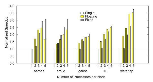
**Figure 4-5.** Baseline system performance comparison. The figure plots application speedups over Single (uniprocessor-node) under Fixed and Floating with increasing number of processors per node. The numbers appearing over the horizontal line at 1 indicate a better performance over Single.
