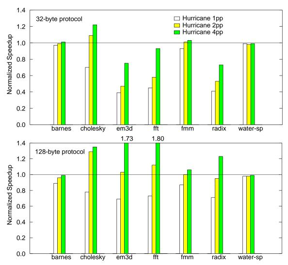
**Figure 5-11.** Impact of block size on Hurricane's performance. The figure compares performance in S-COMA and Hurricane for a 32-byte (above) and a 128-byte (below) block protocol. The graphs plot application speedups in one- (1pp), two- (2pp), and four-processor (4pp) Hurricane systems. The speedups are normalized to S-COMA. Values appearing under the horizontal line at 1 indicate a better performance under S-COMA.
