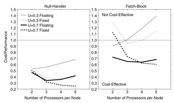
**Figure 4-4.** Relative cost-performance. The figure plots cost-performance of Fixed and Floating ( $O_{int} = 0.5 \ \mu$ s) against varying the number of processors per node for two values of compute-utilization (U = 0.3 and U = 0.7). Costups and speedups are calculated with respect to a uniprocessor node (Single). The graphs assume that the cost of a processor is 30% of the cost of a uniprocessor node. Values over the horizontal line at 1 indicate design points that are not cost-effective.
