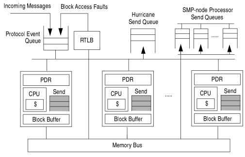
**Figure 5-3.** The Hurricane custom device. The device contains two or more protocol processors, each with a protocol dispatch register, a Typhoon-like block buffer, and a message send queue. The processors share an RTLB which holds the fine-grain access control tags for cached remote data. There is also a message send queue for every compute processor on the node, and a parallel protocol dispatch queue recording block access faults and incoming messages on the node
