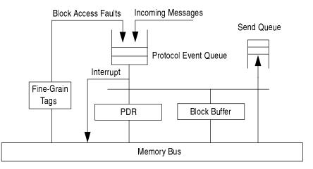
**Figure 4-1.** The Typhoon-1 network interface. The network interface contains a protocol dispatch register, a block buffer, and a message send queue. There is a single SRAM device maintaining the fine-grain tags for cached remote data, and a protocol dispatch queue recording block access faults and incoming messages on the node.
