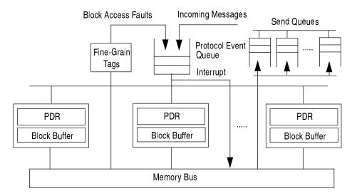
**Figure 5-4.** The Hurricane-1 custom device. The device contains two or more pairs of protocol dispatch registers and Typhoon-like block buffers, and a message send queue per processor on the node. There is a single SRAM device maintaining the fine-grain tags for cached remote data, and a parallel protocol dispatch queue recording block access faults and incoming messages on the node.
