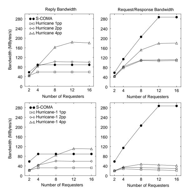
**Figure 5-5.** Protocol bandwidth in S-COMA, Hurricane, and Hurricane-1. The four figures compare S-COMA's reply (left) and request/response bandwidth (right) bandwidth with those in Hurricane (above) and Hurricane-1 (below) for a 64-byte protocol.
