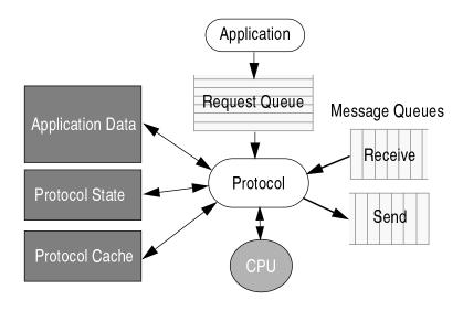
Figure 2-1. Resources for a simple fine-grain software protocol.
