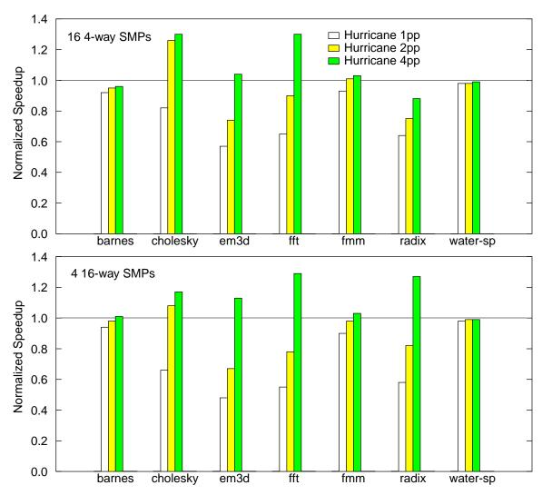
**Figure 5-9.** Impact of clustering degree on Hurricane's performance. The figure compares performance in S-COMA and Hurricane on a cluster of 16 4-way SMPs (above), and a cluster of 4 16-way SMPs (below). The graphs plot application speedups in one- (1pp), two- (2pp), and four-processor (4pp) Hurricane systems. The speedups are normalized to S-COMA. Values appearing under the horizontal line at 1 indicate a better performance under S-COMA.
