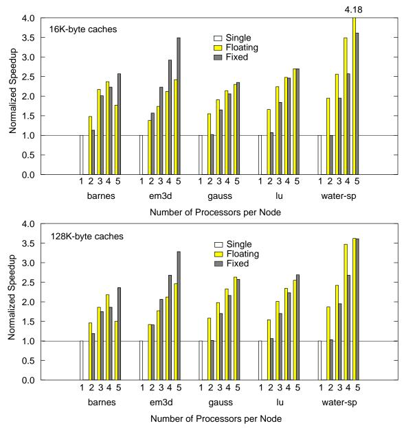
**Figure 4-7.** Performance sensitivity to processor cache size. The figure plots application speedups over Single under Fixed and Floating with increasing number of processors per node for 16-Kbyte processor caches (above) and 128-Kbyte processor caches (below). The numbers appearing over the horizontal line at 1 indicate a better performance over Single.
