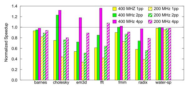
**Figure 5-13.** Impact of protocol processor clock rate on Hurricane's performance. The figure compares Hurricane's performance with 400-MHz and 200-MHz protocol processors on a cluster of 8 8-way SMPs. The graphs plot application speedups normalized to S-COMA for one-, two-, and four-processor Hurricane devices. Values appearing under the horizontal line at 1 indicate a better performance under S-COMA.
