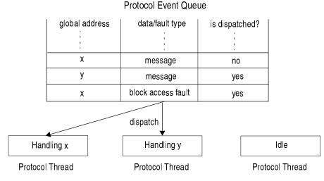
Figure 2-2. Parallel protocol event dispatch in fine-grain DSM.
