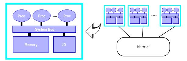
Figure 1-1. Architecture of a cluster of SMPs.
