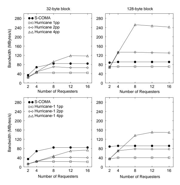
**Figure 5-6.** Impact of block size on protocol reply bandwidth. The figures plot reply bandwidth for a 32-byte (left) and a 128-byte (right) protocol for Hurricane (above) and Hurricane-1 (below).
