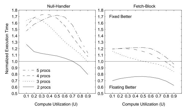
**Figure 4-3.** Relative performance with varying number of processors/node. The figure compares execution times of Fixed and Floating against thread compute-utilization (*U*). The graphs plot Floating's execution time normalized to Fixed for various number of processors per node ( $O_{int} = 0.5 \ \mu$ s). Values over the horizontal line at 1 indicate a better performance under the Fixed policy.
