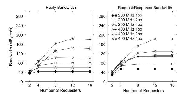
**Figure 5-7.** Impact of processor clock rate on Hurricane's protocol bandwidth. The two figures plot the reply bandwidth (left) and the request/response bandwidth (right) for one-, two-, and four-processor Hurricane devices for current generation (400MHz) and previous generation (200MHz) processor clock speeds.
