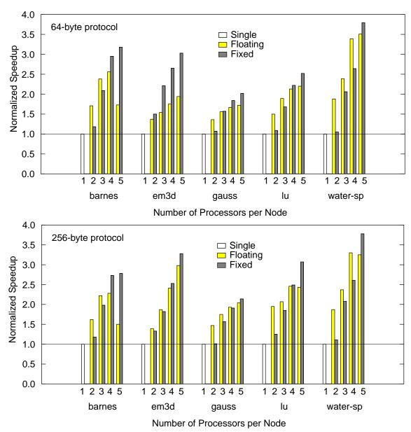
**Figure 4-6.** Performance sensitivity to protocol block size. The figure plots application speedups over Single under Fixed and Floating with increasing number of processors per node for a 64-byte protocol (above) and 256-byte protocol (below). The numbers appearing over the horizontal line at 1 indicate a better performance over Single.
