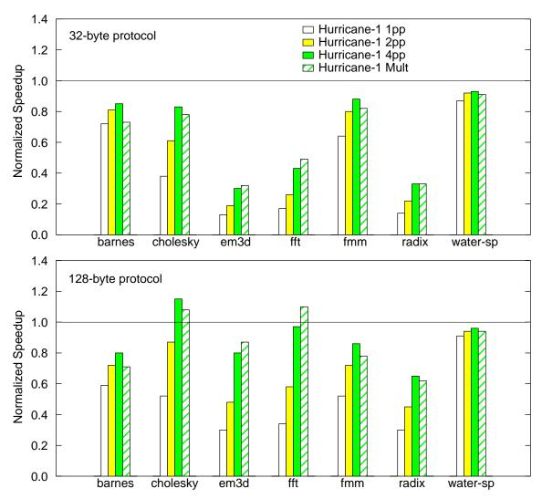
**Figure 5-12.** Impact of block size on Hurricane-1's performance. The figure compares performance in S-COMA and Hurricane-1 for a 32-byte (above) and a 128-byte (below) block protocol. The graphs plot application speedups in one- (1pp), two- (2pp), and four-processor (4pp) Hurricane-1, and Hurricane-1 Mult systems. The speedups are normalized to S-COMA. Values appearing under the horizontal line at 1 indicate a better performance under S-COMA.
