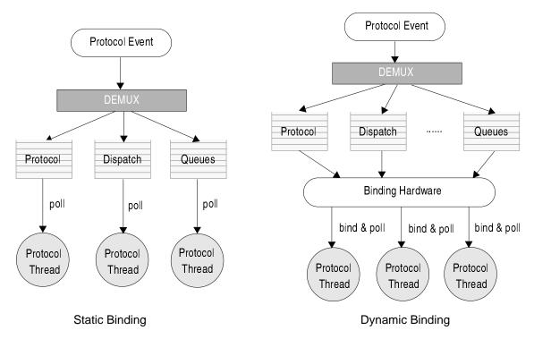
**Figure 2-3.** Static protocol event demultiplexing: protocol events can be both statically demultiplexed and bound (left) or statically demultiplexed and dynamically bound (right) to protocol threads.
