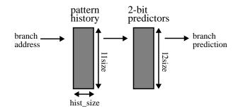
Figure 6. 2-level adaptive predictor structure
