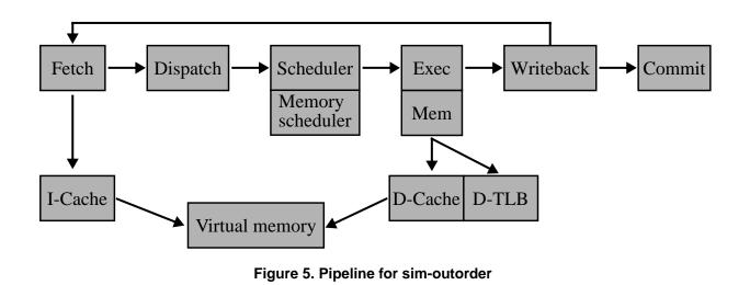
completes). After fetching the instructions, it places them in the dispatch queue, and probes the line predictor to obtain the correct cache line to access in the next cycle.
