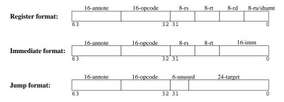
Figure 3. SimpleScalar architecture instruction formats
