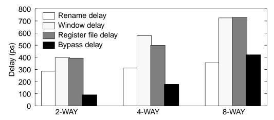
**Figure 2-36.** Overall delay results. This figure shows overall delay results for a 2-way, a 4-way, and a 8-way machine in 0.18µm technology. The 2-way machine has a 48-entry register file and a 16-entry window. The 4-way machine has a 80-entry register file and a 32-entry window. The 8-way machine has a 120-entry register file and a 64-entry window.
