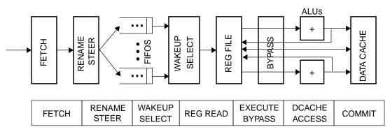
Figure 3-2. Fifo-based microarchitecture.
