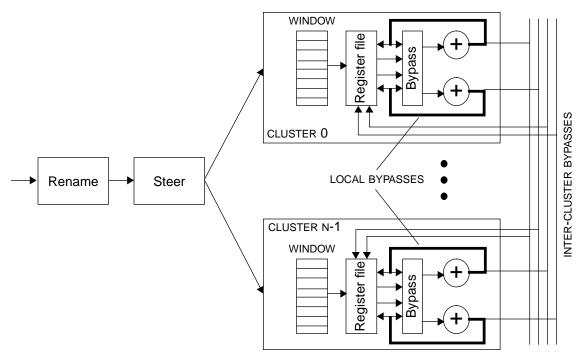
Figure 3-1. Dependence-based superscalar microarchitecture.
