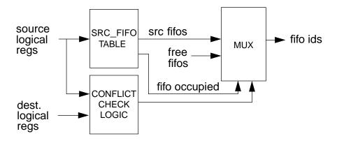
Figure 3-11. Fifo steering hardware.
