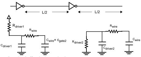
Figure 2-30. Inserting buffers in the result wires.
