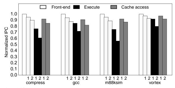
**Figure 2-35.** Effect of pipelining on IPC. This figure shows the effect of pipelining on the performance of a 8-way out-of-order microarchitecture. Each pair of bars shows the effect of introducing one (1) and two (2) extra pipestages in that particular section. The leftmost bar for each benchmark shows the base performance. The simulated processor has a 64-entry window, a 120-entry register file, and a gshare branch predictor with 20 bits of global history.
