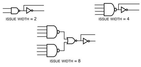
Figure 2-15. Logic for ORing individual match signals.
