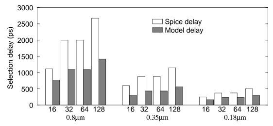
**Figure 2-24.** Model delay results for selection logic. This graph shows how the model delay results compare to the Spice results for selection logic.
