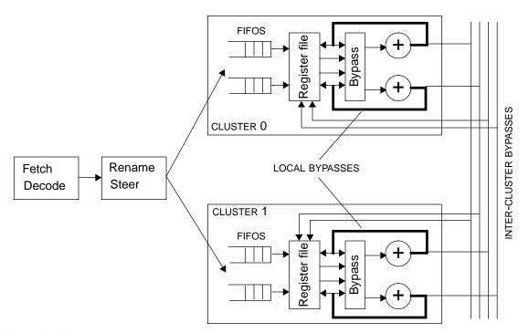
Figure 3-6. Fifo-based microarchitecture with two clusters.
