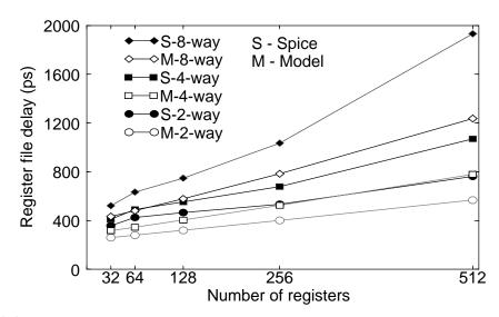
**Figure 2-27.** Model delay results for register file logic. This graph shows how the model delay results compare to the Spice results for 0.18µm technology.
