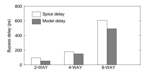
**Figure 2-32.** Model delay results for bypass logic. This graph shows how the model delay results compare to the Spice results for bypass logic implemented in 0.18µm technology.
