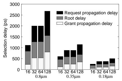
**Figure 2-23.** Selection delay versus window size. This graph shows how the selection delay varies with window size for the three different feature sizes. The selection policy used is based on the location of the instruction in the window.
