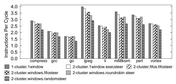
Figure 3-12. Performance of dependence-based superscalar microarchitectures.
