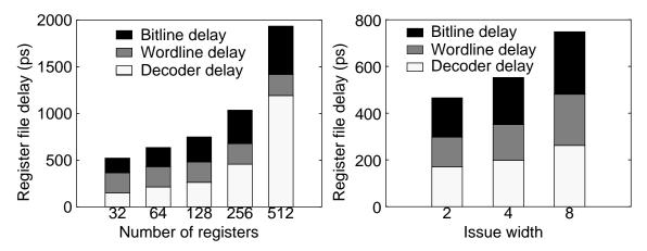
**Figure 2-26.** Breakup of register file delay. The graph on the left shows how the breakup varies with the number of registers for a 8-way machine in 0.18µm technology. The graph on the right shows how the breakup varies with issue width for a 128-entry register file in 0.18µm technology.
