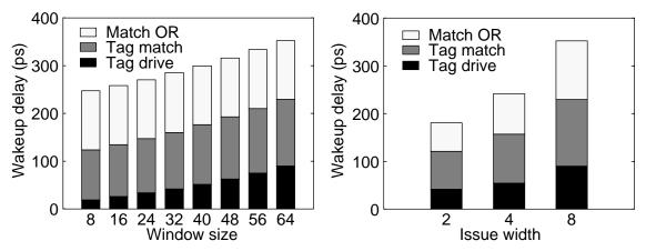
**Figure 2-17.** Wakeup logic delay. The graph on the left shows how wakeup delay varies with window size for a 8-way machine. The graph on the right shows how wakeup delay varies with issue width for a 64-entry window. Both graphs are for 0.18µm technology.
