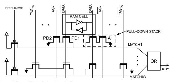
Figure 2-12. CAM cell in wakeup logic.
