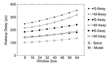
**Figure 2-19.** Model delay results for wakeup logic. This graph shows how the model delay results compare to the Spice results for 0.18µm technology.
