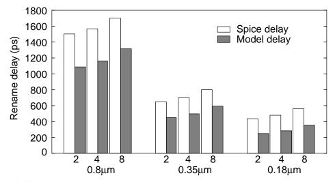
**Figure 2-10.** Model delay results for rename logic. This graph shows how the model delay results compare to the Spice results for register rename logic.
