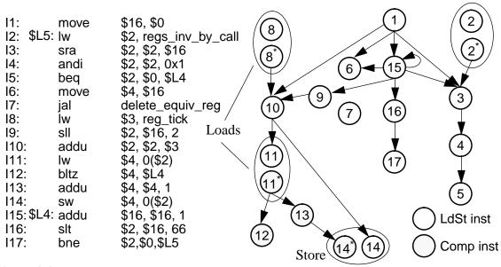
Figure 4-4. Static dependence graph for example program.
