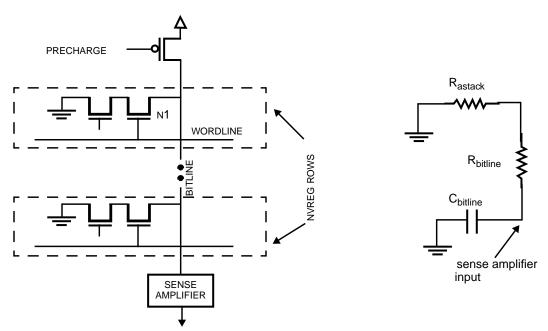
**Figure 2-8.** Bitline structure and equivalent circuit. We used Wada's sense amplifier [WRP92].
