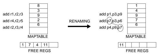
**Figure 2-4.** Renaming example showing dependency checking. The first entry of the map table corresponds to logical register r1.
