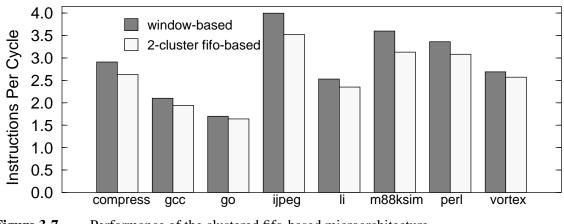
Figure 3-7. Performance of the clustered fifo-based microarchitecture.
