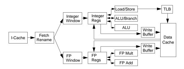
Figure 1-1. A typical superscalar microarchitecture.
