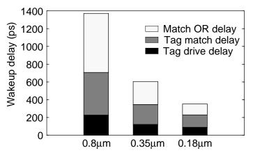
**Figure 2-18.** Wakeup delay versus feature size. This graph shows how the wakeup delay for a 8-way machine with a 64-entry window varies with feature size.
