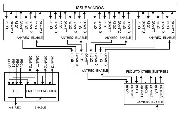
**Figure 2-20.** Selection logic. This figure shows the arbiter tree of the selection logic and a single arbiter cell in detail.
