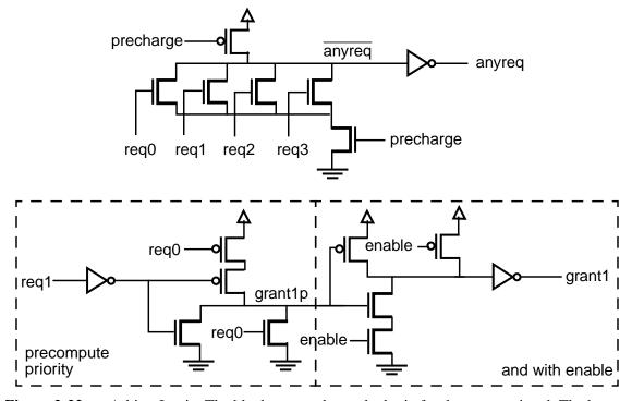
**Figure 2-22.** Arbiter Logic. The block on top shows the logic for the *anyreq* signal. The bottom block shows the logic for generating the *grant1* signal.
