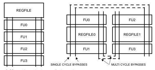
Figure 2-33. Alternative layouts for bypassing.
