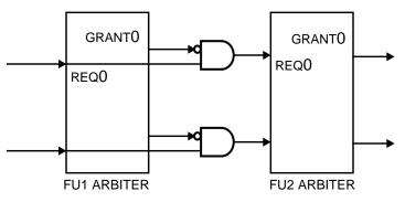
Figure 2-21. Handling multiple functional units.
