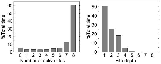
**Figure 3-5.** Fifo utilization. The graph on the left shows the number of active fifos during the execution of *m88ksim*. The graph on the right shows the depth of a particular fifo during the execution of the program.
