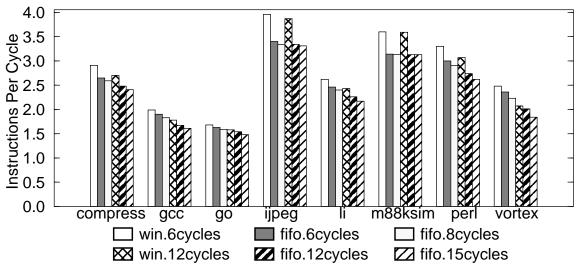
Figure 3-9. Effect of Scaling Instruction and Data Cache Miss Latency.
