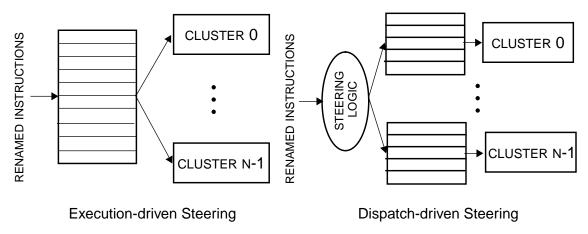
Figure 3-10. Other dependence-based microarchitectures.
