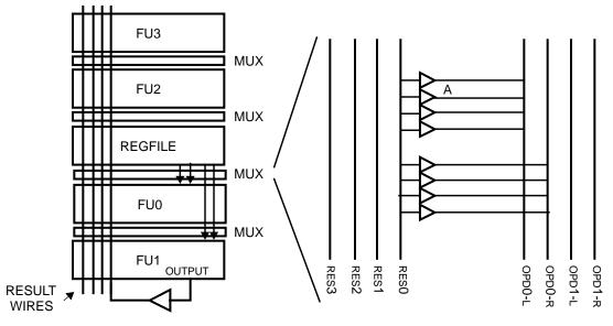
Figure 2-28. Bypass logic.
