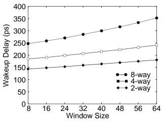
**Figure 2-16.** Wakeup logic delay versus window size. This graph shows how the delay of the window wakeup logic varies with window size and issue width for 0.18µm technology.
