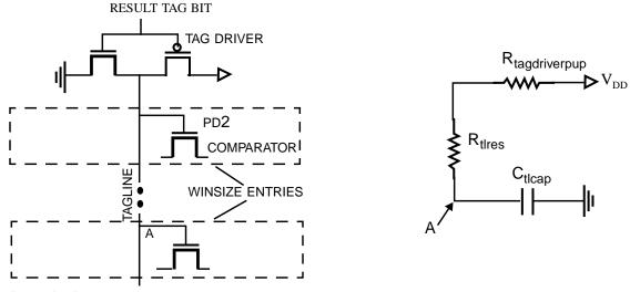
Figure 2-13. Tag drive structure.
