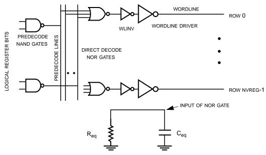
Figure 2-6. Decoder structure and equivalent circuit.
