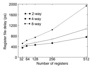
**Figure 2-25.** Register file logic delay. This graph shows how the delay of the register file implemented in 0.18µm varies with issue width and the number of registers
