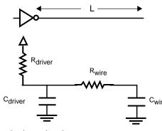
Figure 2-29. Bypass logic equivalent circuit.
