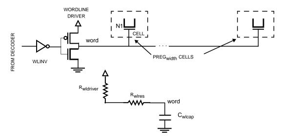
Figure 2-7. Wordline structure and equivalent circuit.
