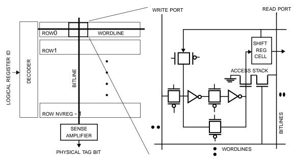
**Figure 2-5.** Rename map table. This figure shows the map table of the rename logic on the left and a single cell of the map table on the right.
