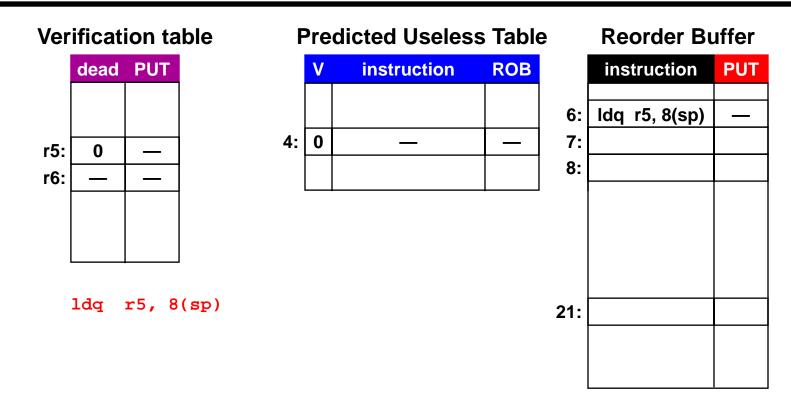
Add VT (verification table) to track prediction status Add PUT (predicted useless table) to enable recovery Augment ROB with pointers into PUT
