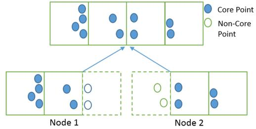
Figure 7: Example of the second type of merge where a core point detected by one node is being detected as a non-core point in a neighboring node. This case is caused by a shadow region not having all neighbor points available (furthest left and furthest right grid cells shown).
