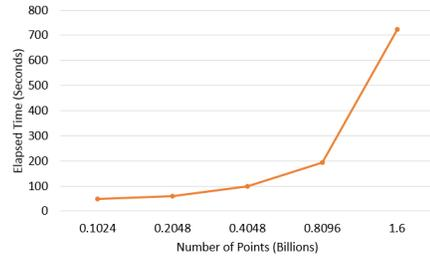
Figure 13: Elapsed partitioning time for Mr. Scan for the SDSS dataset
