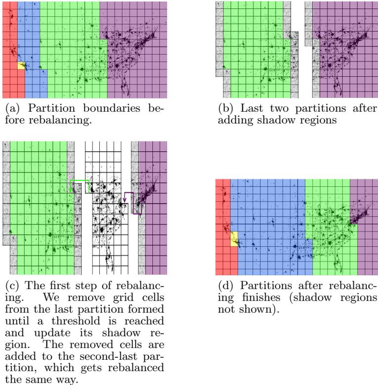
Figure 2: Mr. Scan’s partition algorithm
