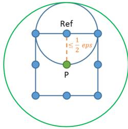
Figure 5: Any overlapping core point  $P$  must be within  $\frac{1}{2} \times Eps$  of at least one corner or side of the grid cell. We label this point  $Ref$ . This means that the representative point for  $Ref$  must fall within a  $\frac{1}{2} \times Eps$ -neighborhood of  $Ref$ . Since this entire region (shown as the blue circle) is contained in the  $Eps$ -neighborhood of  $P$  this means that  $P$  is always within  $Eps$  of a representative point.
