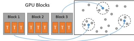
Figure 3: CUDA-DClust GPGPU blocks expanding seed points [6].
