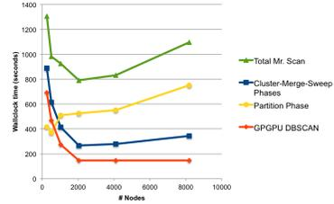
Figure 10: Elapsed time of Mr. Scan when clustering 6.5 billion points and varying the number of cluster processes.
