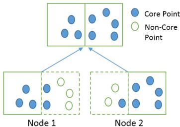
Figure 6: Example of a core point overlap between clusters detected on different nodes.
