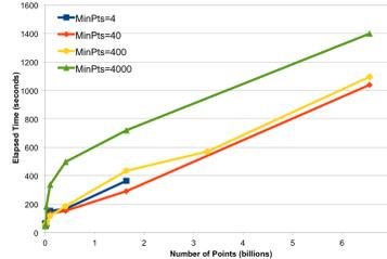
Figure 8: Elapsed time of Mr. Scan for the configurations listed in Table 1. *Eps*=0.1 and *MinPts* varies as indicated.
