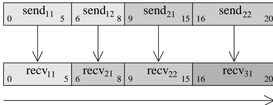
**b:** Partitioning message-passing operations into fragments to establish one-to-one mapping between the fragments. A fragment marked  $\text{send}_{ij}$  or  $\text{recv}_{ij}$  represents the  $j^{\text{th}}$  fragment of the original operation  $\text{send}_i$  or  $\text{recv}_i$ .
