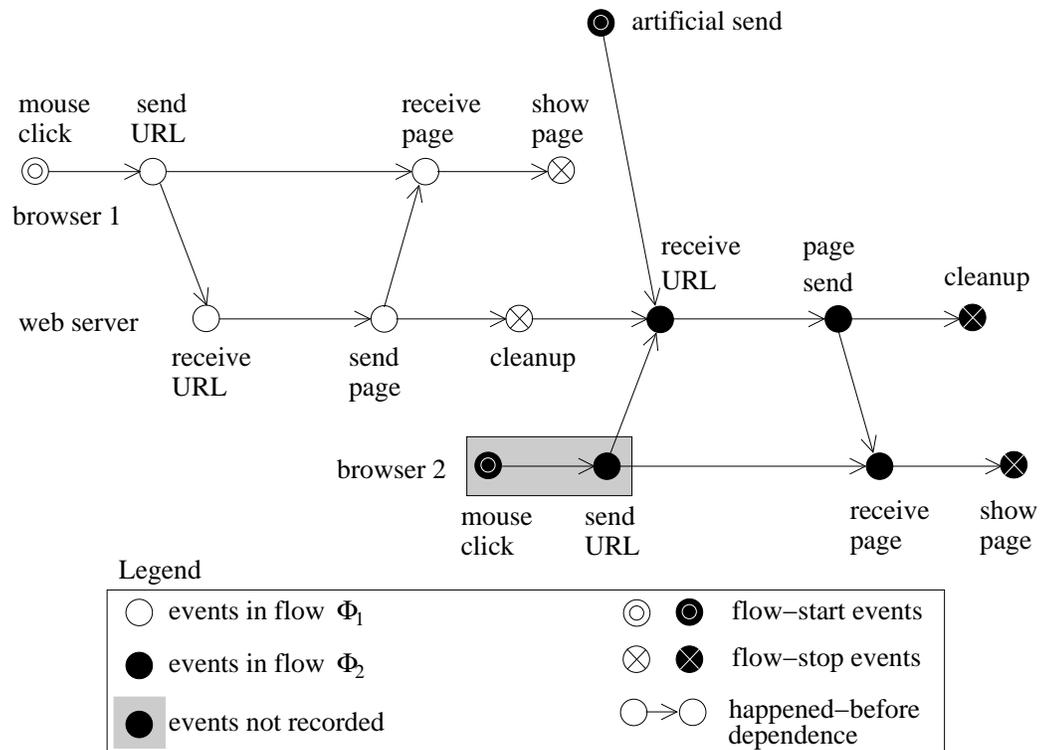
**Figure 4.7:** *The PDG for a Web server that executes requests from two browsers. The user identified only one start event, from flow  $\Phi_1$ . Events from flow  $\Phi_2$  in the Web server are recorded but the corresponding start event is not. We detect this situation and introduce an artificial send event for flow  $\Phi_2$ .*
