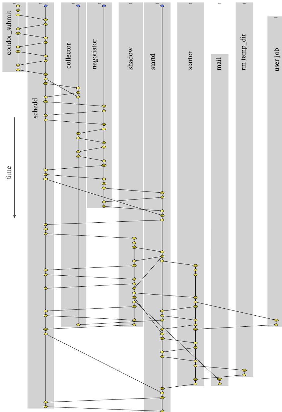
**Figure 6.13:** A simplified flow graph for processing a Condor job. Gray rectangles represent timelines of processes. Dots in a rectangle represent communication events.
