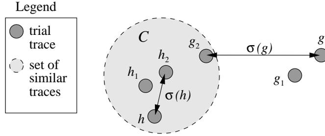
**Figure 5.2:** *Computing the suspect scores  $\sigma(g)$  and  $\sigma(h)$  for an anomalous trace  $g$  and normal trace  $h$ .  $C$  is a large collection of traces with similar behaviors;  $g_i$  and  $h_i$  are the  $i^{\text{th}}$  trial neighbors of  $g$  and  $h$  respectively.*
