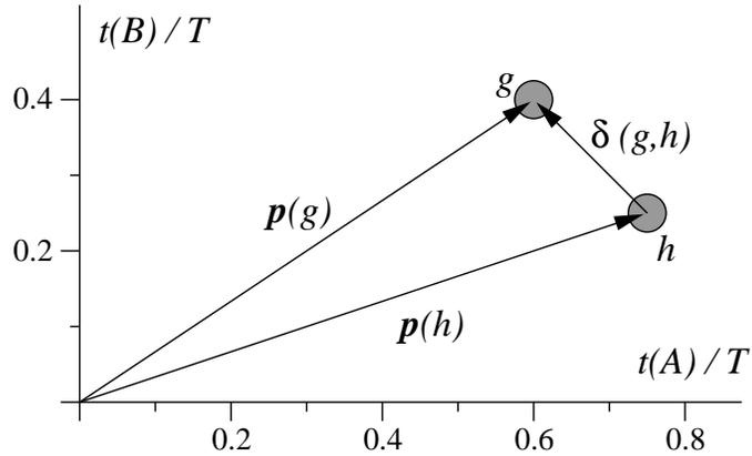
**Figure 5.1:** The two data points correspond to processes  $g$  and  $h$  with profile vectors  $\mathbf{p}(g)$  and  $\mathbf{p}(h)$ . The coordinates of the points are determined by the relative contributions  $t(A)$  and  $t(B)$  of functions  $A$  and  $B$  to the total time  $T$  in each process.  $\delta(g, h)$  is the difference vector between  $\mathbf{p}(g)$  and  $\mathbf{p}(h)$ .
