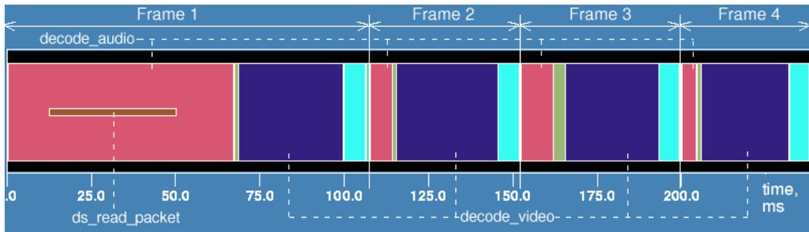
**Figure 6.3:** *A user-level trace of MPlayer showing functions called directly from main and the anomalous call to ds\_read\_packet*
