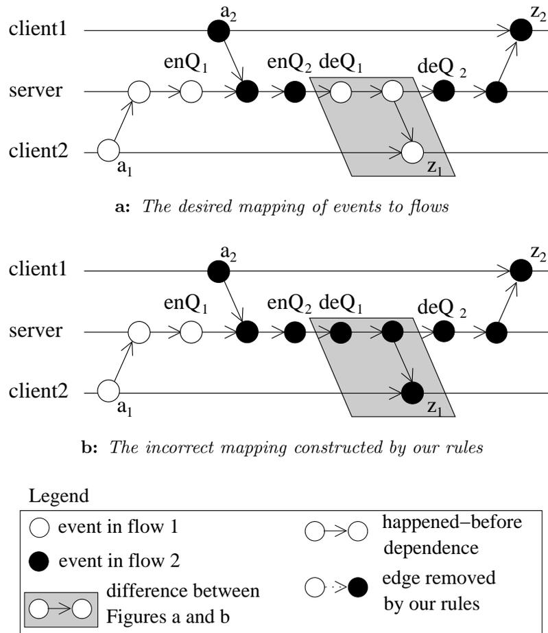
**Figure 4.8:** *The PDG for a system that uses a queue to hold and process incoming requests. Events  $enQ_i$  and  $deQ_i$  correspond to enqueueing and dequeueing request  $i$ .*
