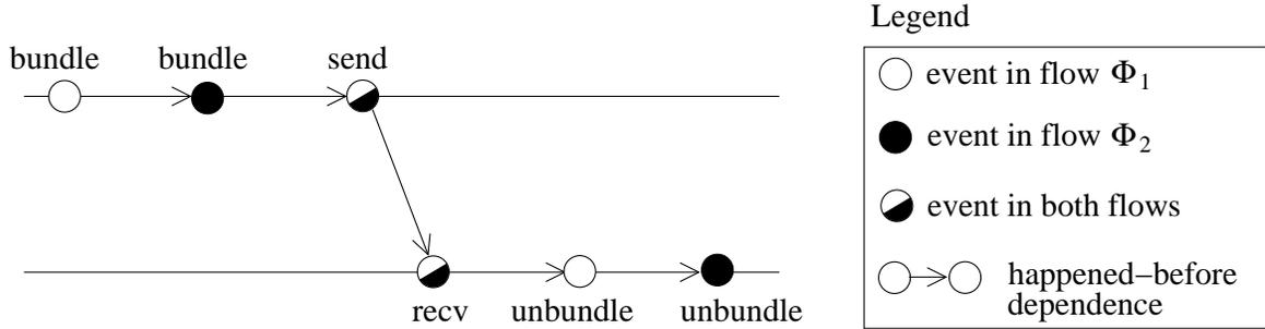
**Figure 4.4:** *The PDG for a system that uses message bundling. The `send` and `recv` events belong to both requests and violate Flow Property 4.*
