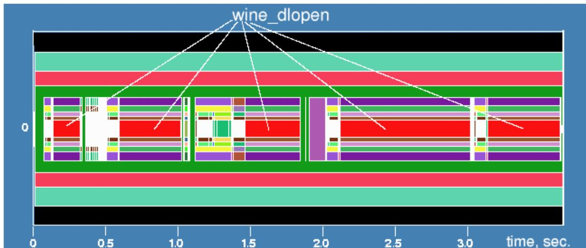
**Figure 6.6:** Trace of functions on opening a drop-down menu (low-level details hidden)
