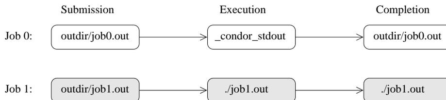
**Figure 6.15:** Output file names at job submission, execution, and completion phases. White boxes represent the names for the first job. Gray boxes represent the names for the second job.
