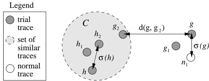
**Figure 5.3:** Computing the suspect scores  $\sigma(g)$  and  $\sigma(h)$  where both  $g$  and  $h$  are normal, but  $g$  is unusual;  $n_1$  is the closest normal neighbor of  $g$ .
