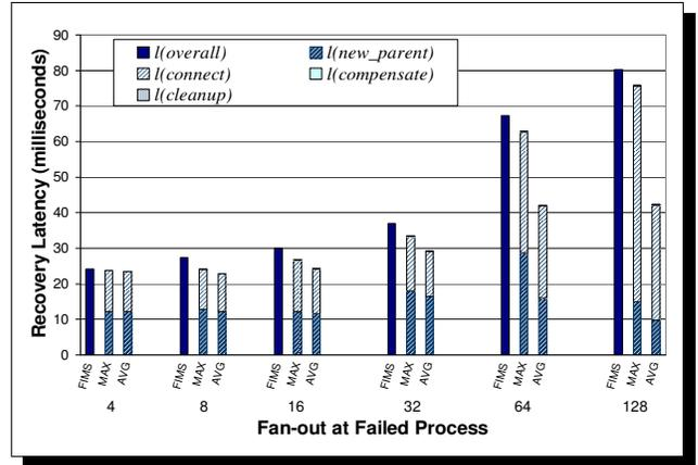
Figure 6. Recovery Latencies:  $l(overall)$  is overall TBÖN recovery estimate,  $l(new\_parent)$ ,  $l(connect)$ ,  $l(compensate)$  and  $l(cleanup)$  are the times to choose parent, connect, send filter state, and do cleanup.
