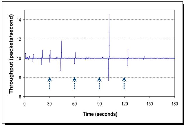
Figure 7. Application Perturbation: Failures (indicated by arrows) are injected every 30 seconds into a TBON with an initial 32<sup>3</sup> topology.
