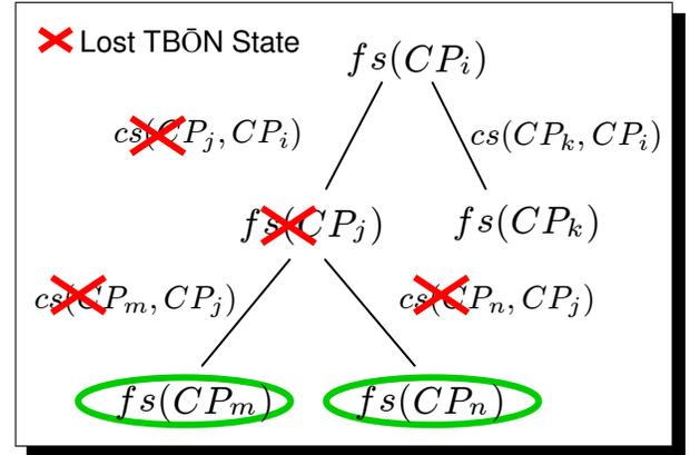
Figure 4. State Composition: When  $CP_j$  fails,  $fs(CP_j)$ ,  $cs(CP_j, CP_i)$ ,  $cs(CP_m, CP_j)$ , and  $cs(CP_n, CP_j)$  are lost.  $fs(CP_m)$  and  $fs(CP_n)$  compensate for the loss.
