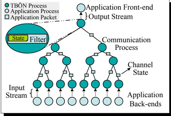
Figure 1. TBON Model: back-ends stream data via communication processes that aggregate and propagate the data to the front-end.
