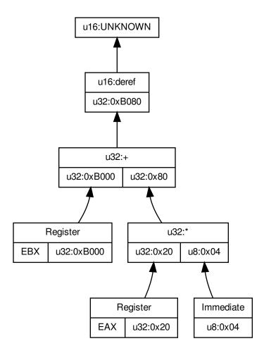
Figure 6: Applying eval to a Dereference tree with two registers having user-provided values.
