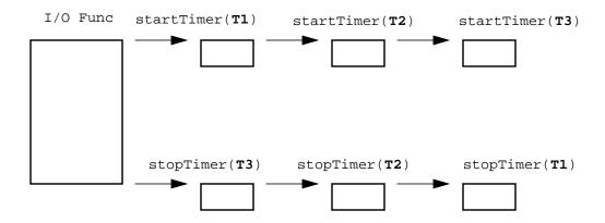
Notice that T3 gets the best placement for being inserted last. Meanwhile, T1 gets the worst placement after being inserted first. As new timers are inserted, the earlier timers get less and less accurate because they must also time *all* the new timers' instrumentation.
