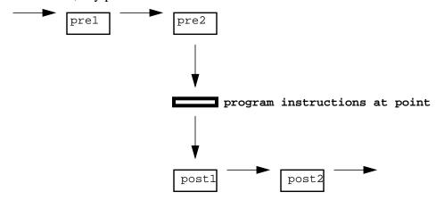
You should try to avoid using entry-point post-instrumentation because the program instructions found at the point may be branch instructions. These instructions will divert execution flow away from the post-instrumentation, as illustrated in the figure below. When this happens, any post-instrumentation will not be executed. In practice, we have not found it necessary to use entry-point post-instrumentation.
