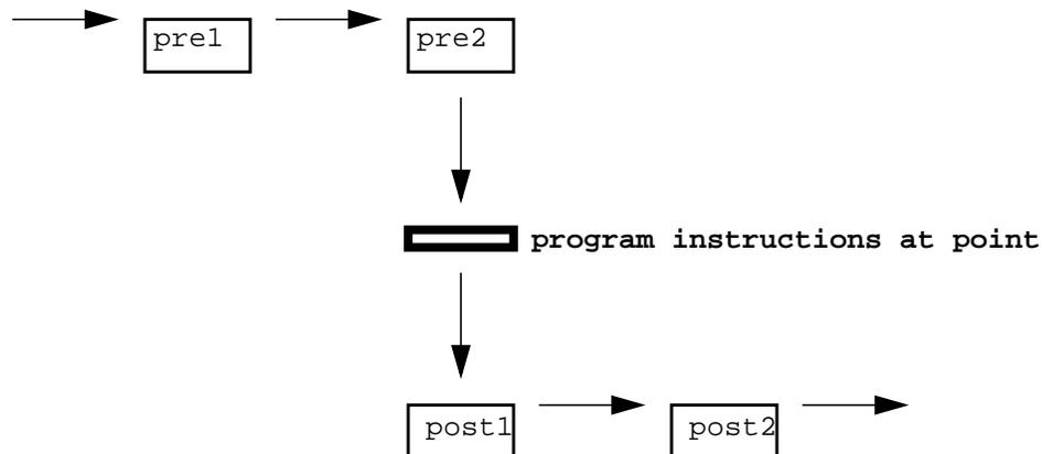
You should try to avoid using entry-point post-instrumentation because the program instructions found at the point may be branch instructions. These instructions will divert execution flow away from the post-instrumentation, as illustrated in the figure below. When this happens, any post-instrumentation will not be executed. In practice, we have not found it necessary to use entry-point post-instrumentation.
