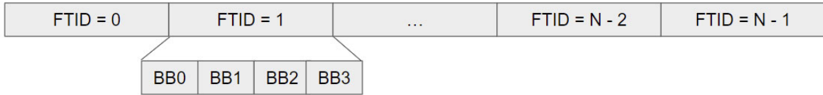
Figure 5: Example Heap Layout for kernels with 4 basic blocks
