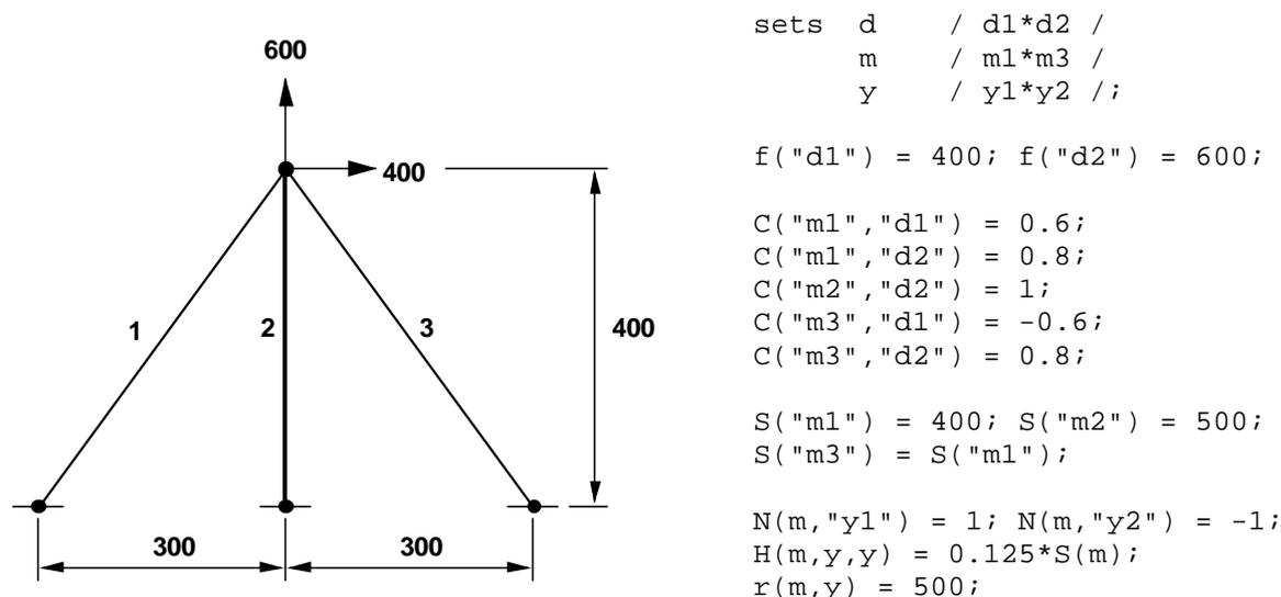
Figure 2: Three-bar truss and associated `state.dat` input
