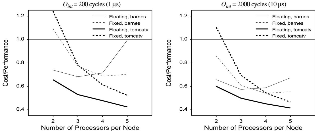
**FIGURE 7. Cost-performance of Fixed and Floating with varying number of processors**
