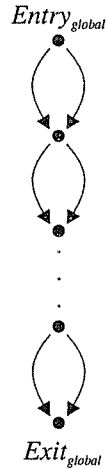
Figure 19: Schematic of a graph where the number of paths from Entry_{global} to Exit_{global} is exponential in the number of nodes in the graph.
