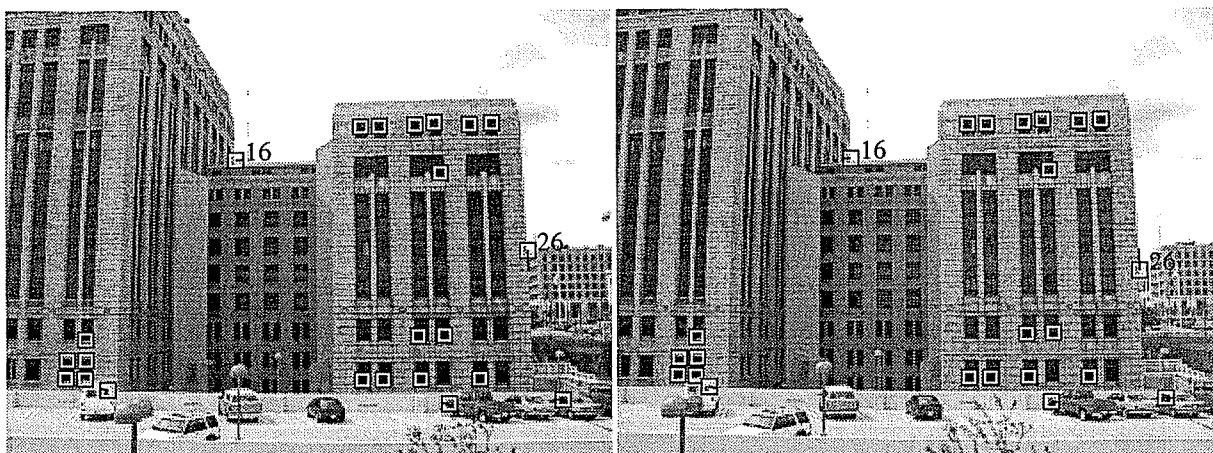
Figure 6.2: Example of false features . Features #16 and #26 are caused by a depth discontinuity and do not represent rigid points in the scene. Instead, their apparent 3D position changes with viewpoint. False features are difficult to detect because their projected image motion is smooth and similar to that of rigid feature points.
