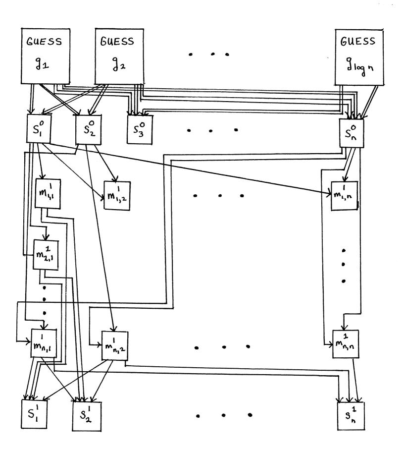
First Level of Circuit to Test Whether  $G_{H_1}$  generates  $H_1$
