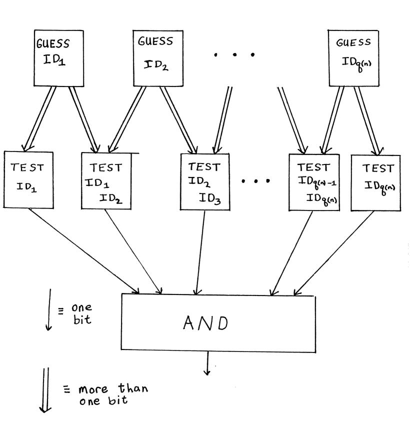
of M. Most of the work is done by the *test* subcircuits. If the first ID is correct, each tester is satisfied, and the state of the last ID is a final state the circuit accepts, otherwise it rejects. Since the final AND-circuit has q(n) inputs, it is easy to build an NC circuit to do this computation.
