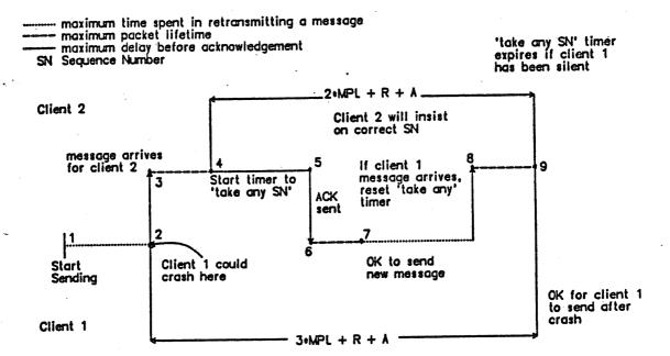
When a message has arrived at a server handler but has not yet been accepted, the requester kernel will issue periodic probing messages to the server kernel. If no response is heard after retransmissions in the interval MPL +  $\Delta t$ , the requester kernel will report to its client that the server is dead. Similarly, when a REQUEST or an ACCEPT is issued and no response is heard after retransmitting during the interval MPL +  $\Delta t$ , the destination is reported dead.
