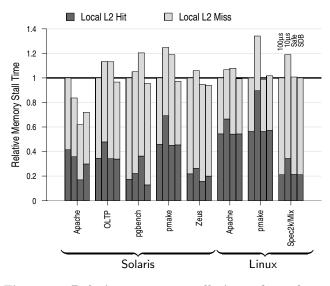
Figure 3: Relative memory stall time of synchronization management techniques. Four bars for each benchmark (from left to right) represents results for a 100 $\mu$ s timeslice, 10 $\mu$ s timeslice, safe point aware preemption and SDB, respectively. Results are normalized to the 100 $\mu$ s timeslice (lower is better).
