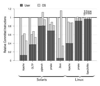
Figure 2: Relative instruction counts of synchronization management techniques. Four bars for each benchmark (from left to right) represents results for a 100 $\mu$ s timeslice, 10 $\mu$ s timeslice, safe point aware preemption and SDB. Results are normalized to the 100 $\mu$ s timeslice (lower is better).
