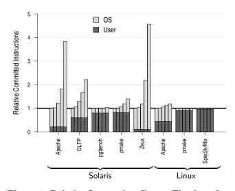
Figure 1: Relative Instruction Count. Five bars for each benchmark (from left to right) represent results for  $10\mu$ s,  $20\mu$ s,  $50\mu$ s,  $100\mu$ s and  $200\mu$ s timeslices. Results are normalized to the  $10\mu$ s timeslice (lower is better).
