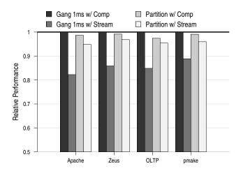
Figure 7: Performance isolation. Bars represent performance when a commercial workload in one VM is paired with a second VM running either a computationally-intensive (*Comp*), or cacheintensive (*Stream*), microbenchmark.
