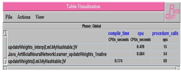
Figure 3: Performance data for the updateWeights method from the dynamically compiled neural network Java application. The table shows the performance measures total CPUTime (second column) and number of calls (third column), for both the byte-code (top row), and native (middle row) forms, and compile time (first column) associated w/the wrapper (bottom row).
