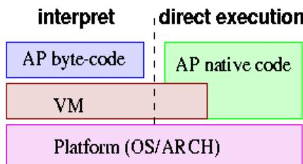
**Figure 1: During a dynamically compiled execution methods may be interpreted by the VM and/or compiled into native code and directly executed. The native code may still interact with the VM. In this case, the VM acts like a runtime library to the AP.**
