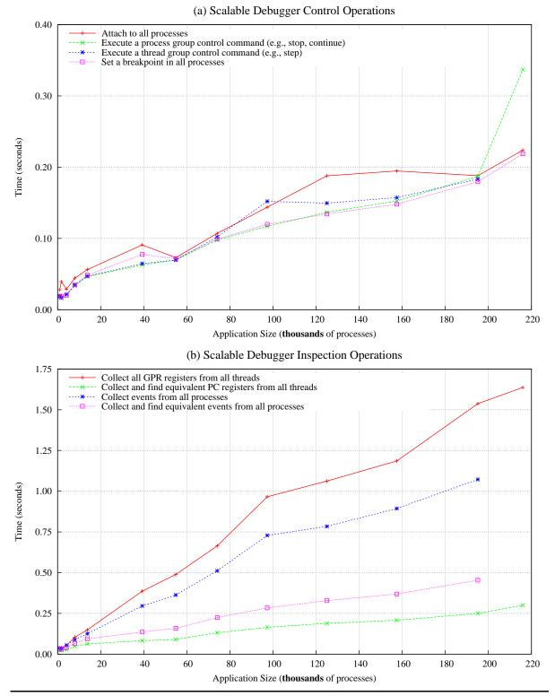
**Figure 6.9 tbon-dbg Group Control and Inspection Operations** Time required to complete common debugging tasks using distributed proc++ files
