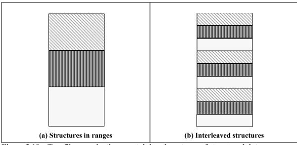
Figure 3.10 Two file organizations containing three types of structured data(a) All structures of a given type reside within a single range.(b) Structures of different types are interleaved.
