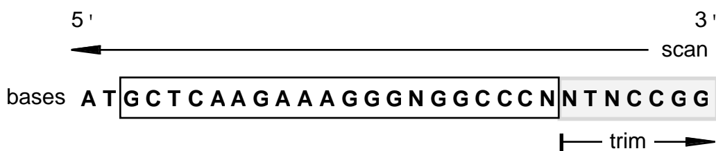
Figure 4-2. N-Trim . The window_size is 20 and max_Ns is two. When scanning from the 3' end, the boxed window is the first to contain two or fewer N s and data in the shaded region is trimmed.
