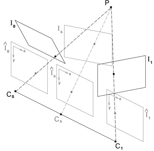
Figure 4: View Morphing in Three Steps. (1) Original images  $\mathcal{I}_0$  and  $\mathcal{I}_1$  are prewarped to form parallel views  $\hat{\mathcal{I}}_0$  and  $\hat{\mathcal{I}}_1$ . (2)  $\hat{\mathcal{I}}_s$  is produced by morphing (interpolating) the prewarped images. (3)  $\hat{\mathcal{I}}_s$  is postwarped to form  $\mathcal{I}_s$ .
