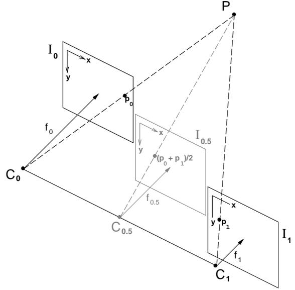
Figure 3: Morphing Parallel Views. Linear interpolation of corresponding pixels in parallel views with image planes  $\mathcal{I}_0$  and  $\mathcal{I}_1$  creates image  $\mathcal{I}_{0.5}$ , representing another parallel view of the same scene.
